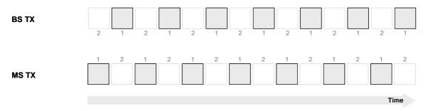
Figure 5.2: Offset channel timing
