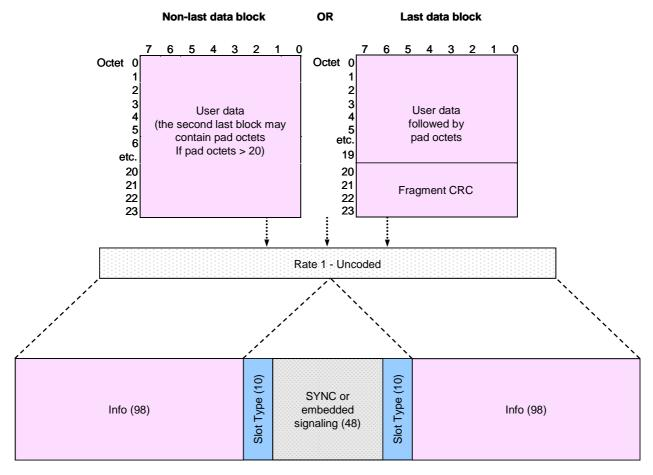
Figure 8.13: Unconfirmed rate 1 coded data block format
