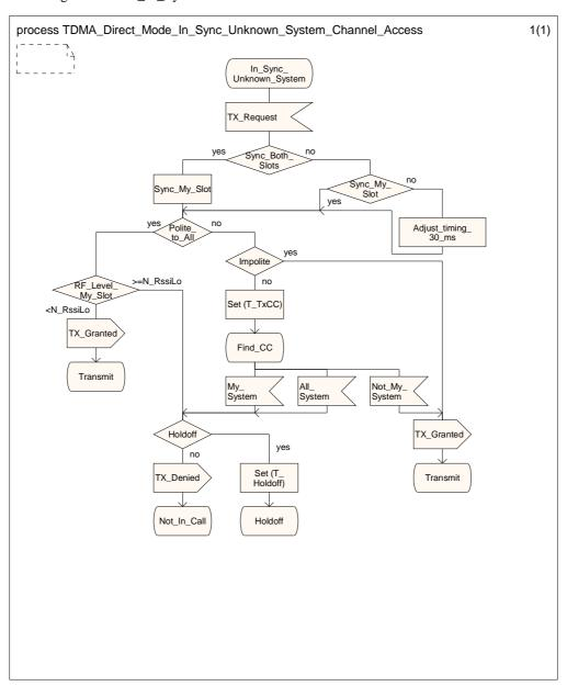
Figure 5.39: In \_Sync\_Unknown\_System SDL diagram
