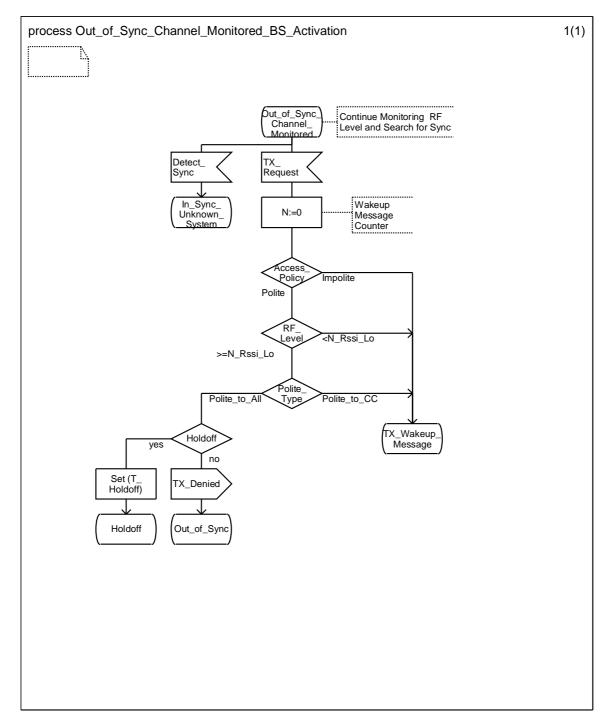
Figure 5.31: Out\_of\_Sync\_Channel\_Monitored channel access
