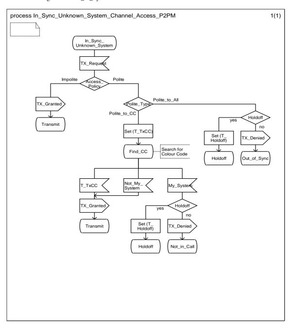
Figure 5.29: In\_Sync\_Unknown\_System SDL diagram
