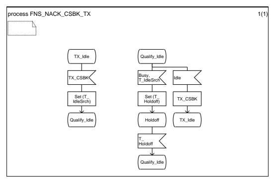
Figure 5.36: FNS channel access SDL diagram
