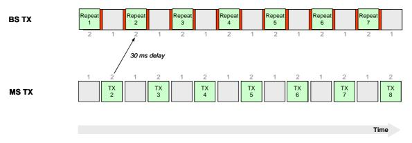
Figure 5.13: Offset channels repeated voice timing - 30 ms delay
