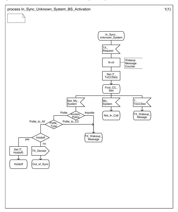
Figure 5.32: In\_Sync\_Unknown\_System SDL diagram
