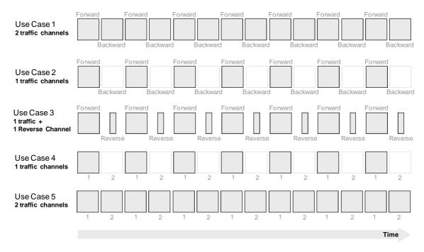
Figure 5.26: Single frequency (bi-directional) channel
