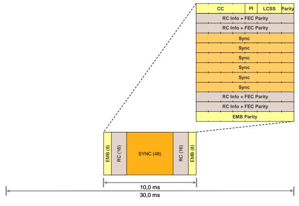
Figure 6.7: Standalone inbound Reverse Channel (RC) burst
