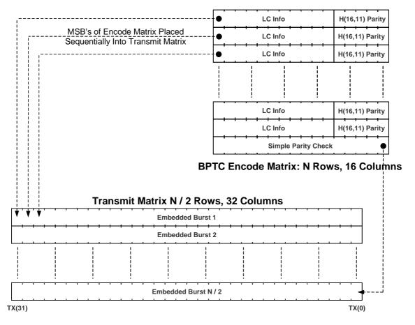
Figure B.2: Format for embedded signalling BPTC
