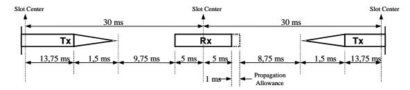
Figure C.1: Direct mode timing diagram
