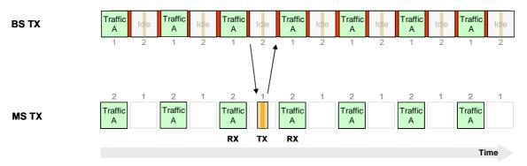
Figure 5.23: Standalone inbound Reverse Channel (RC) timing
