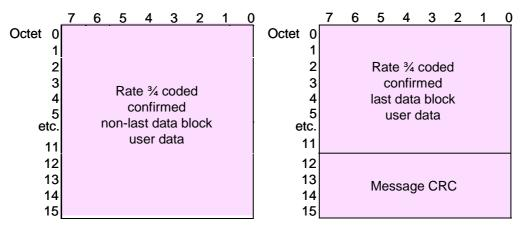
Figure B.8D: Rate 3/4 coded confirmed user data bit numbering
