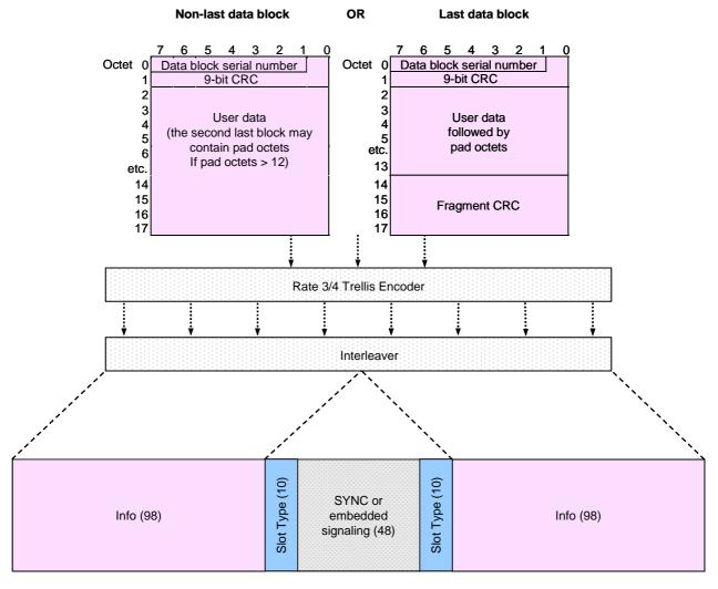
Figure 8.14: Confirmed rate 3/4 coding data block format
