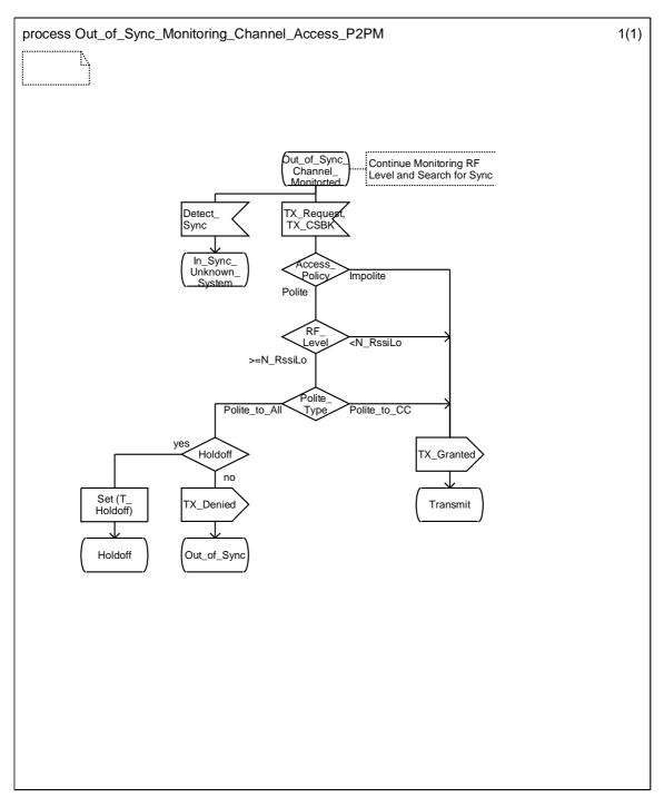
Figure 5.28: Out\_of\_Sync\_Channel\_Monitored SDL diagram
