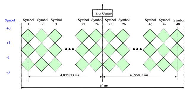
Figure 10.6: Reverse Channel (RC) burst symbol timing within a slot
