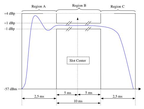
Figure 10.5: Power waveform mask for standalone Reverse Channel (RC) burst
