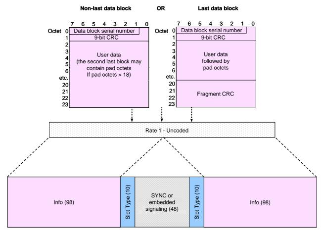
Figure 8.16: Confirmed rate 1 coding data block format
