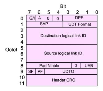
Figure 8.10: Specific first header block for UDT data packet
