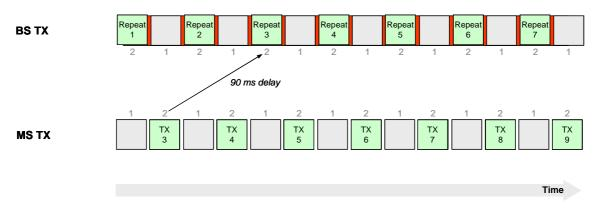
Figure 5.14: Offset channels repeated voice timing - 90 ms delay
