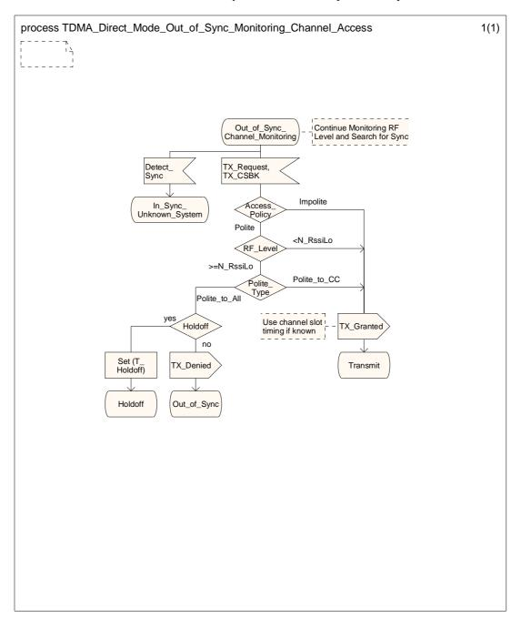
Figure 5.38: Out\_of\_Sync\_Channel\_Monitored SDL diagram
