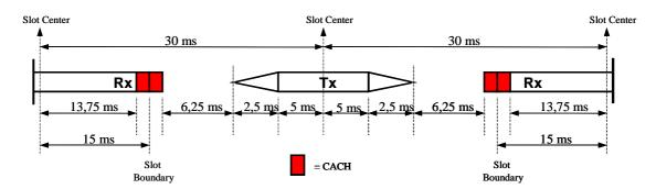
Figure C.2: Reverse Channel timing diagram
