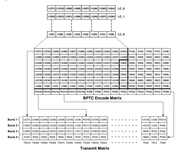
Figure B.3: Format for burst embedded signalling
