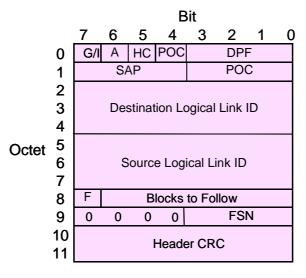
Figure 8.3: Specific first header block for unconfirmed packet
