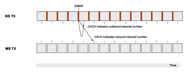
Figure 4.9: CACH channel indicator timing
