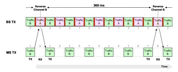
Figure 5.21: Embedded outbound Reverse Channel (RC) timing
