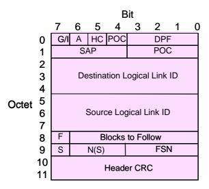
Figure 8.4: Specific first header block for confirmed packet
