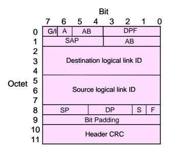
Figure 8.8: Specific first header block for raw short data packet
