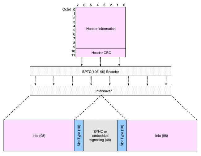
Figure 8.2: Structure of the generic first header block
