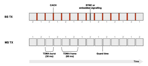
NOTE: The example timing in figure 4.2 applies to a two frequency BS.
