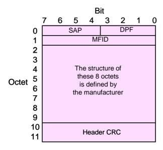
Figure 8.6: Second header block of a proprietary packet
