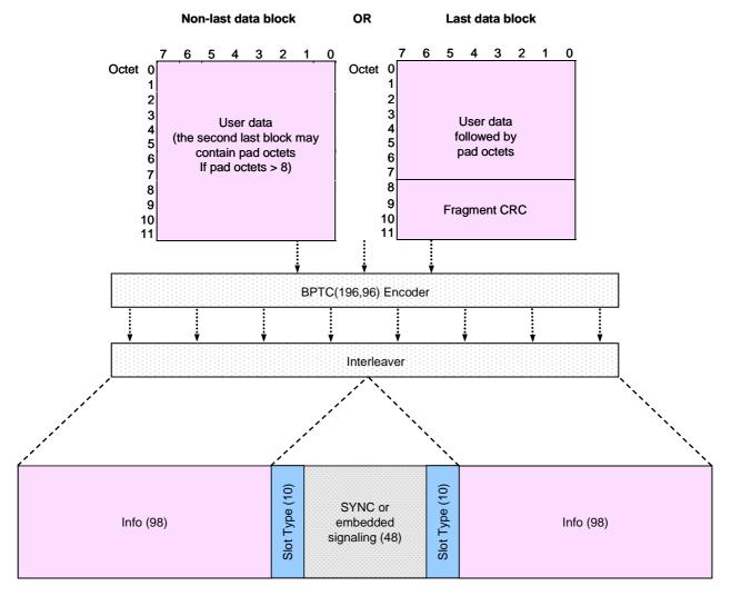
Figure 8.11: Unconfirmed rate ½ coded data block format
