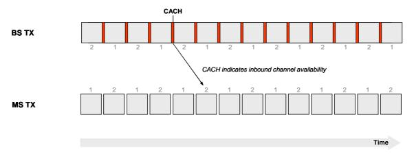
Figure 4.8: Access type indicator timing
