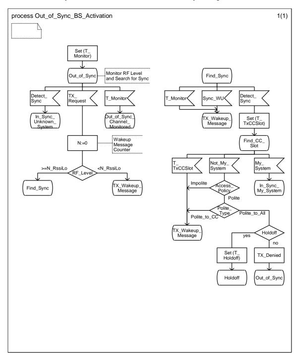
Figure 5.30: Out\_of\_Sync SDL diagram
