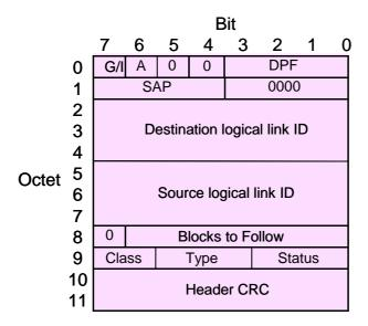
Figure 8.5: Specific first header block for response packet
