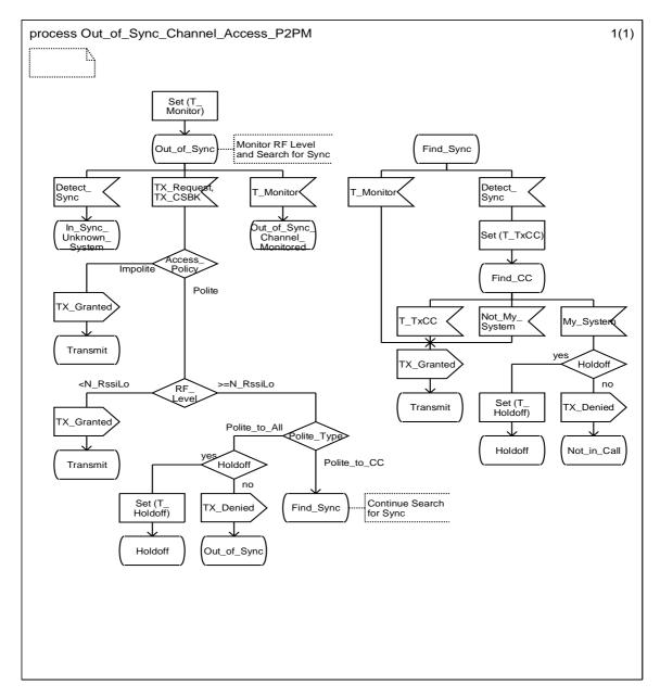
Figure 5.27: Out\_of\_Sync SDL diagram
