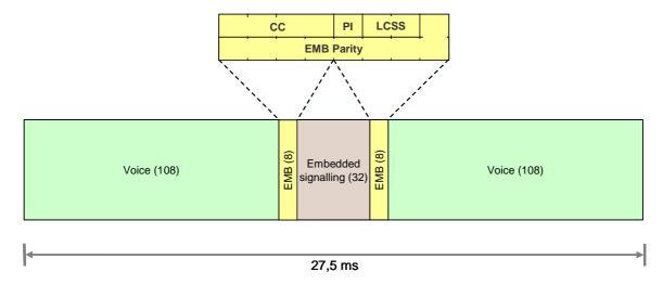
Figure 6.4: Voice burst with embedded signalling
