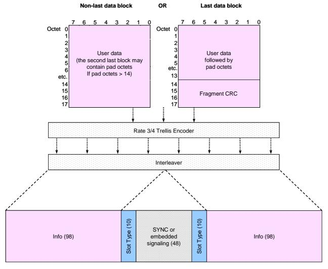
Figure 8.12: Unconfirmed rate ¾ coded data block format
