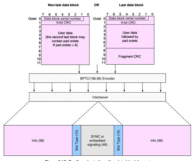
Figure 8.15: Confirmed rate  $\frac{1}{2}$  coding data block format
