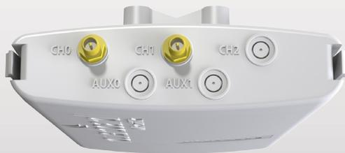
The RB912 is also available in an outdoor enclosure, fit with two SMA connectors for antennas, and a cable hood for protection against moisture. Also available are three additional places for antenna connectors, in case you wish to use the RB912 miniPCIe slot for one more wireless interface to make a dual band device.
